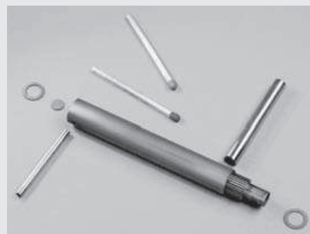
THTMD in parts before laser-welding
