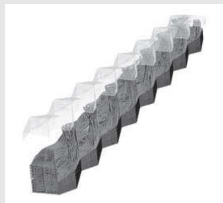
Simulated "real" flow profiles at high flow rates in Caterpillar Micromixers
