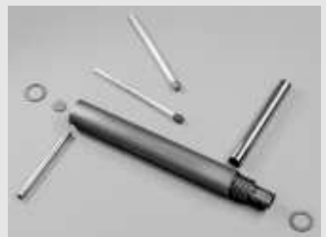
THTMD in parts before laser-welding
