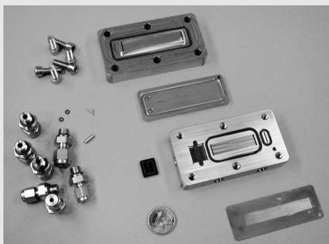
Disassembled Micro Bubble Column MBC
