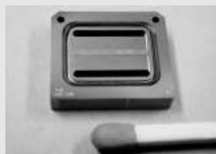
Gas/liquid UV-LIGA contacting unit
