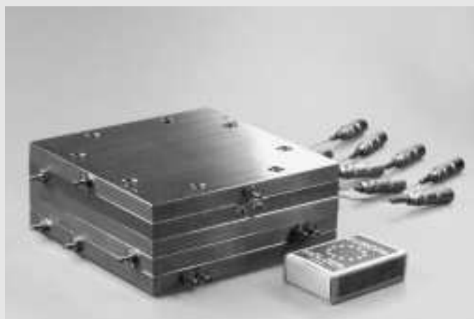
LLMR-SY; a reactor with internal arrangement of 4 LLMR-MIX including delay loop
