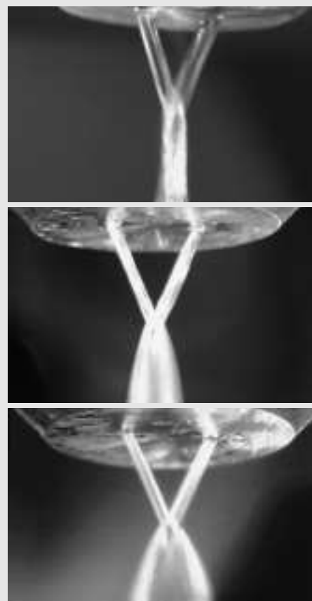
3 different flow patterns: • Y-type jet of IJMM (top) • Fan-shaped jet (middle) • Fanned-out jet (down)
