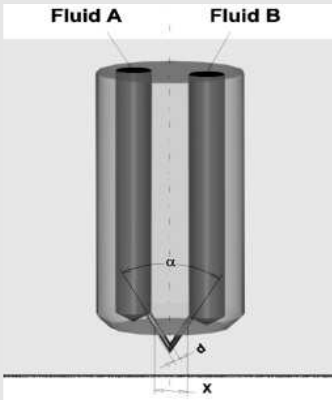
Geometric parameters determine the mixing performance, beside flow parameters
