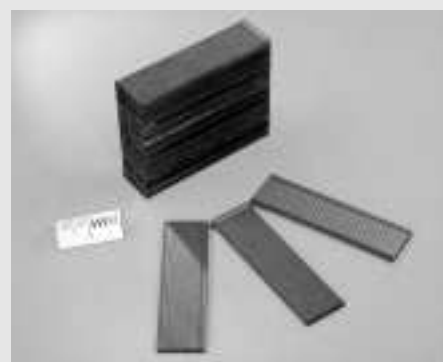
Stack of cartridges with coated microstructured plates
