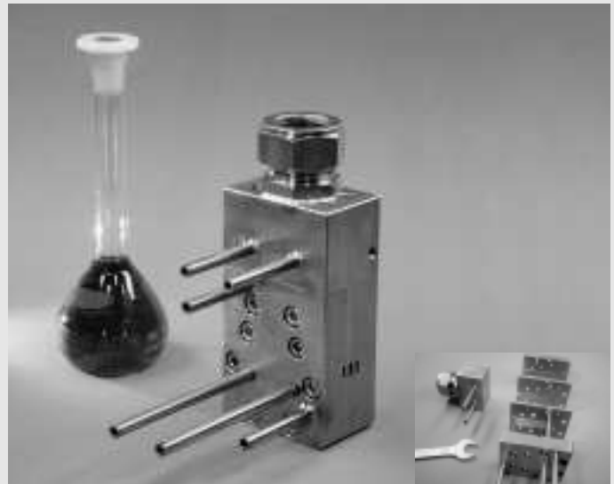
CPMM-R2400/10-HEX-SO-ss-wt assembled with straight outlet connector and integrated heat exchanger
