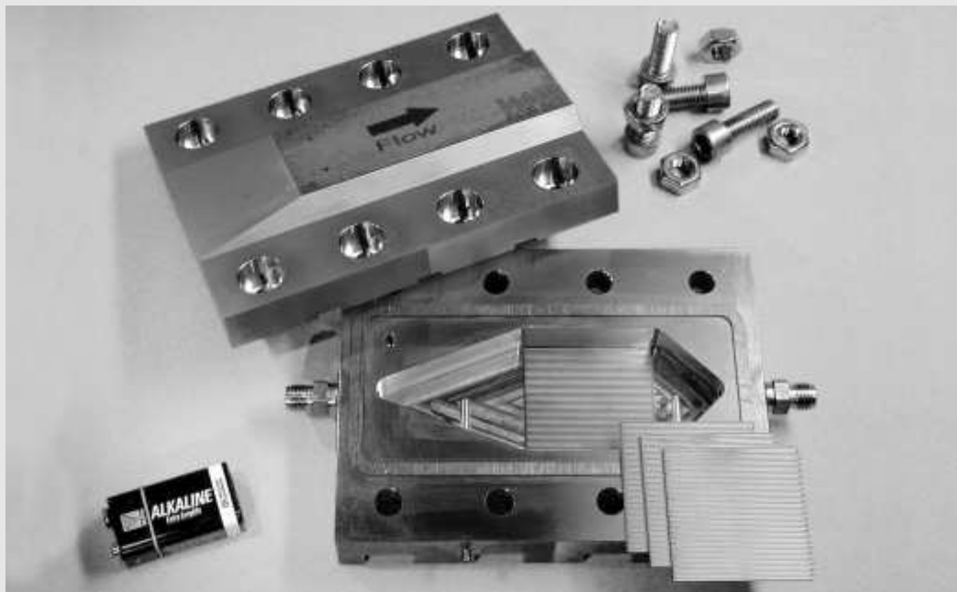
Single parts of the Catalyst Micro Burner Reactor
