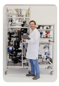
After a promising laboratory development at the labs of Microinnova, a continuously operating manufacturing plant for this reaction has been designed and realized by Microinnova Engineers. The plant has been handed over to the Pharma customer in the Middle East. The modular system consists of 2 feed modules and one complex reaction unit.
